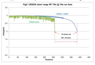
drop allowed the BLE Tx to utilise nearly all the energy in the battery before brown-out, greatly extending battery life. Again, this is due to the reduced voltage droop due to the low supercapacitor ESR.
