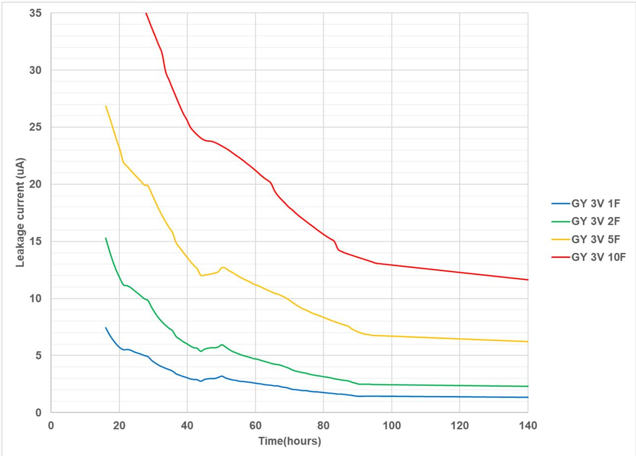
Fig 3: Leakage current measurement
