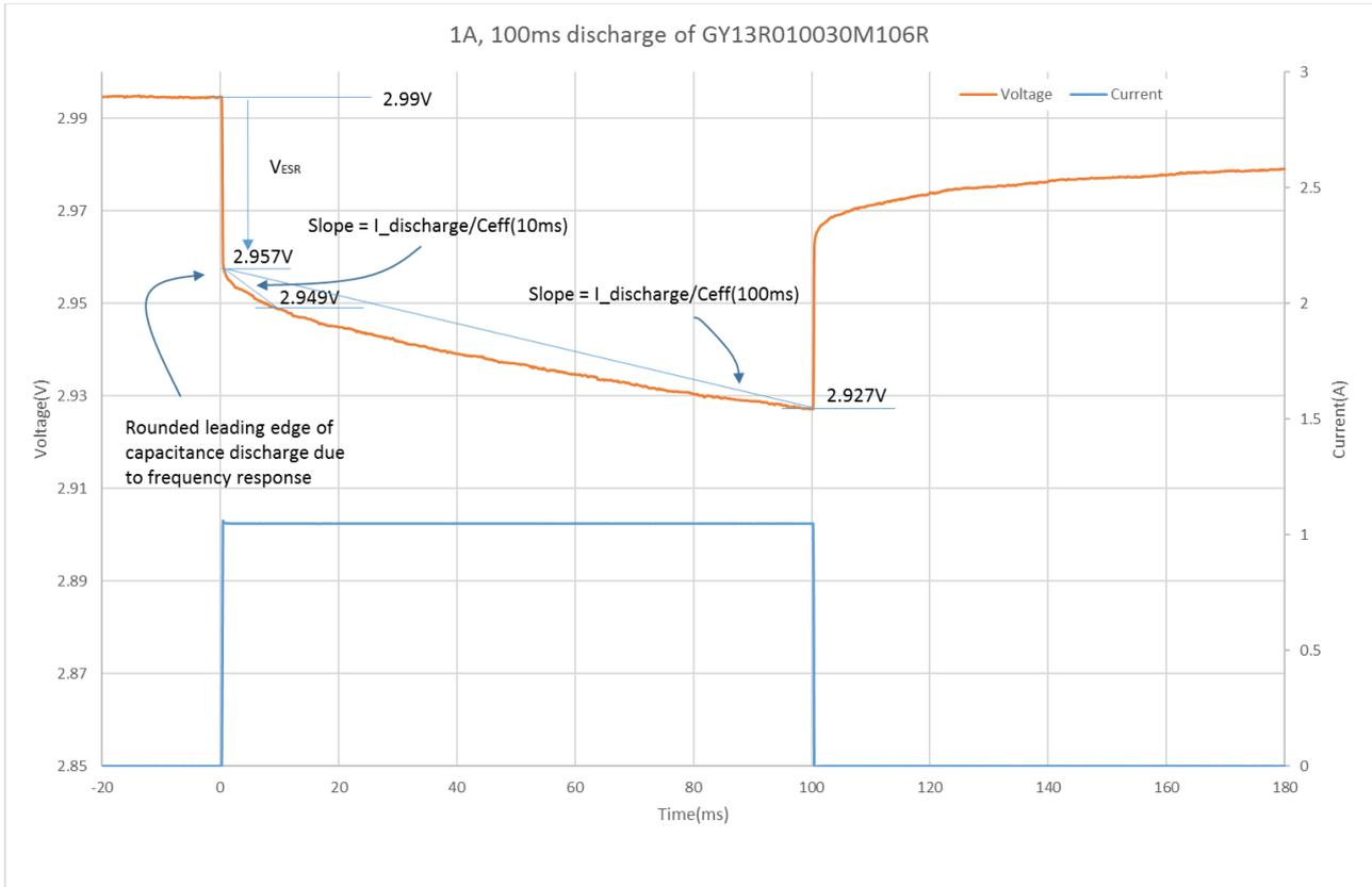
Fig 7: Discharge pulse illustrating the concept of Ceff
