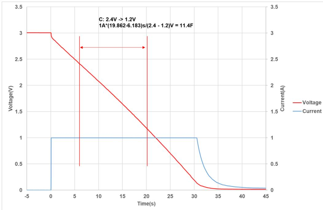
Fig 1: Capacitance measurement
