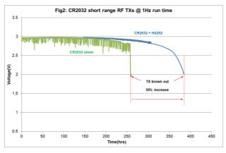
drop allowed the BLE Tx to utilise nearly all the energy in the battery before brown-out, greatly extending battery life. Again, this is due to the reduced voltage droop due to the low supercapacitor ESR.
