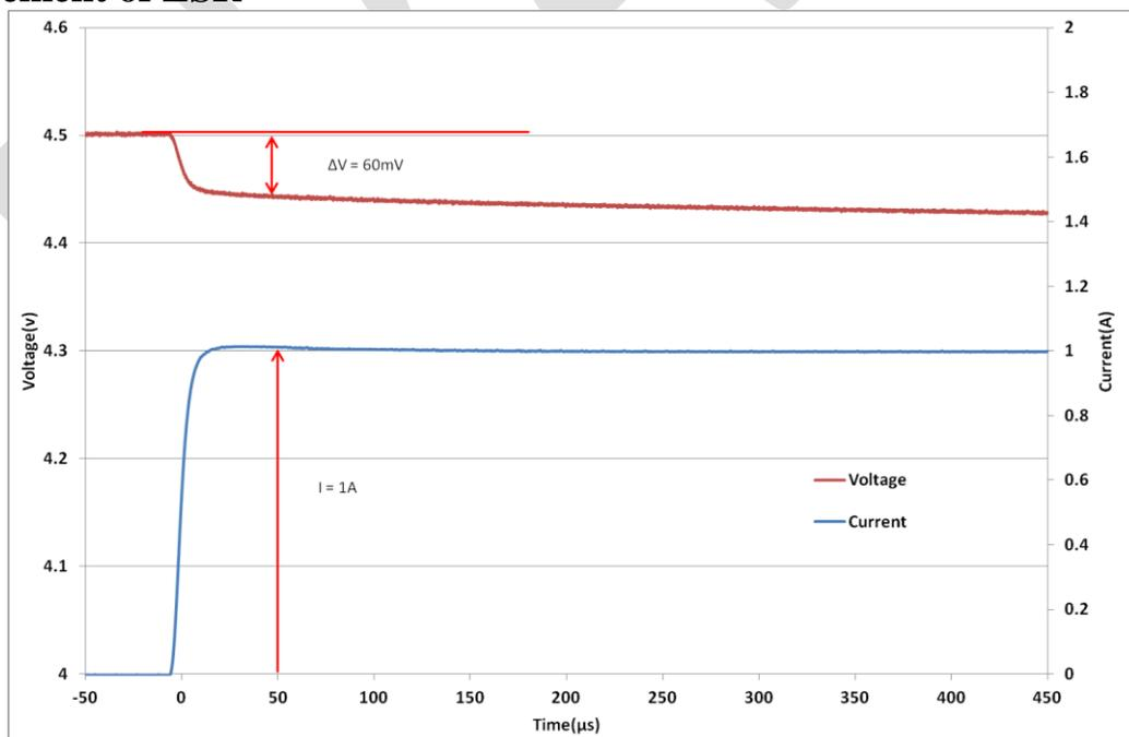
**Fig 3: Measurement of ESR for a GA230**
