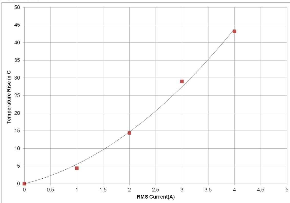
**Fig 12: Temperature rise in GA230 with RMS current**
