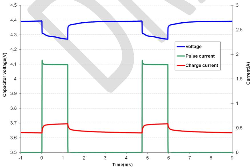
Fig 5 shows that the GA230 supercapacitor does an excellent job supporting a GPRS class 10 pulse train, drawing 1.8A for 1.1ms at 25% duty cycle. The source is current limited to 0.6A and the supercapacitor provides the 1.2A difference to achieve the peak current. At first glance the freq response of Fig 8 indicates the supercapacitor would not support a 1ms pulse, but the  $C_{eff}$  of 40mF coupled with the low ESR supports this pulse train with only ~120mV drop in the supply rail.
