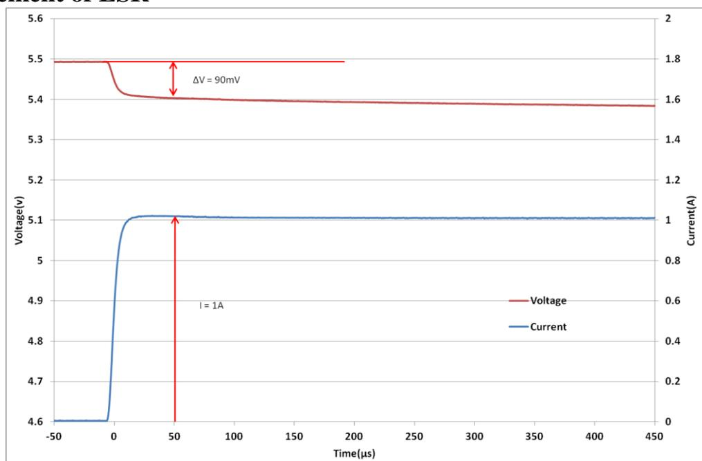
**Fig 3: Measurement of ESR for an HW201**
