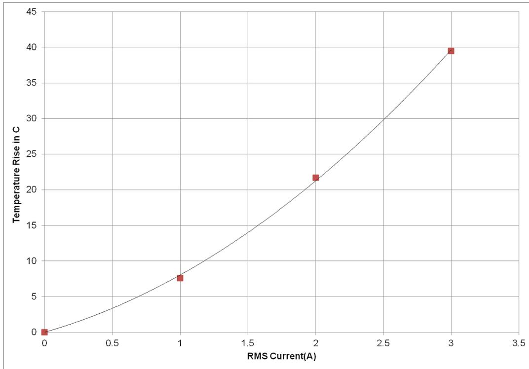
**Fig 12: Temperature rise in HW201 with RMS current**
