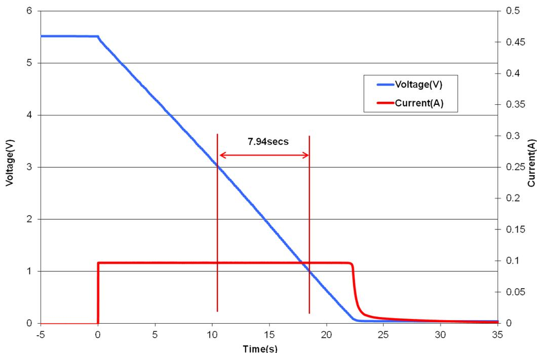
**Fig 2: Measurement of DC Capacitance for an HW201**
