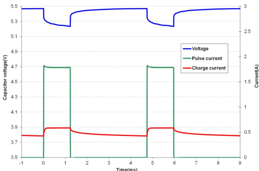
Fig 5 shows that the HW201 supercapacitor does an excellent job supporting a GPRS class 10 pulse train, drawing 1.8A for 1.1ms at 25% duty cycle. The source is current limited to 0.6A and the supercapacitor provides the 1.2A difference to achieve the peak current. At first glance the freq response of Fig 8 indicates the supercapacitor would not support a 1ms pulse, but the  $C_{eff}$  of 34.2mF coupled with the low ESR supports this pulse train with only ~230mV droop in the supply rail.
