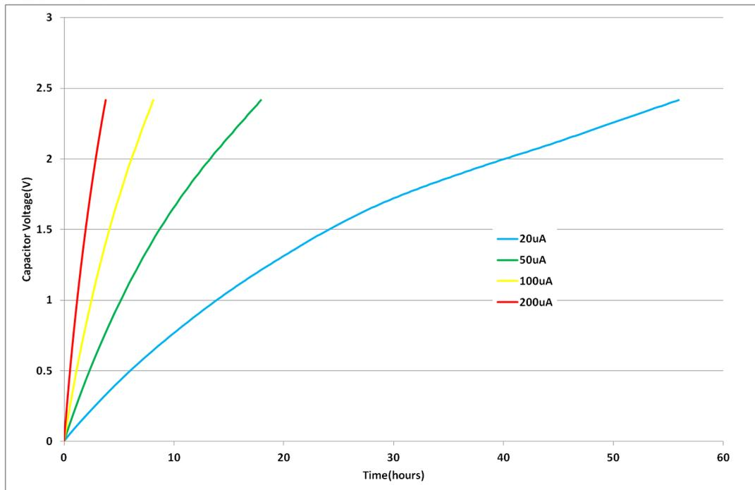
**Fig 11: Charging an HW101 with low current**
