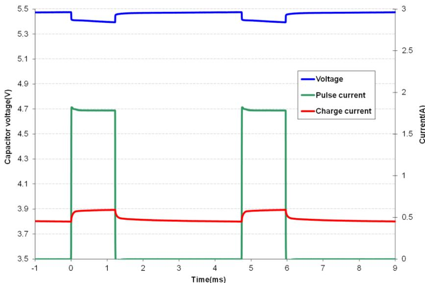
Fig 5 shows that the HS208 supercapacitor does an excellent job supporting a GPRS class 10 pulse train, drawing 1.8A for 1.1ms at 25% duty cycle. The source is current limited to 0.6A and the supercapacitor provides the 1.2A difference to achieve the peak current. At first glance the freq response of Fig 8 indicates the supercapacitor would not support a 1ms pulse, but the  $C_{eff}$  of 72mF coupled with the low ESR supports this pulse train with only ~80mV droop in the supply rail.
