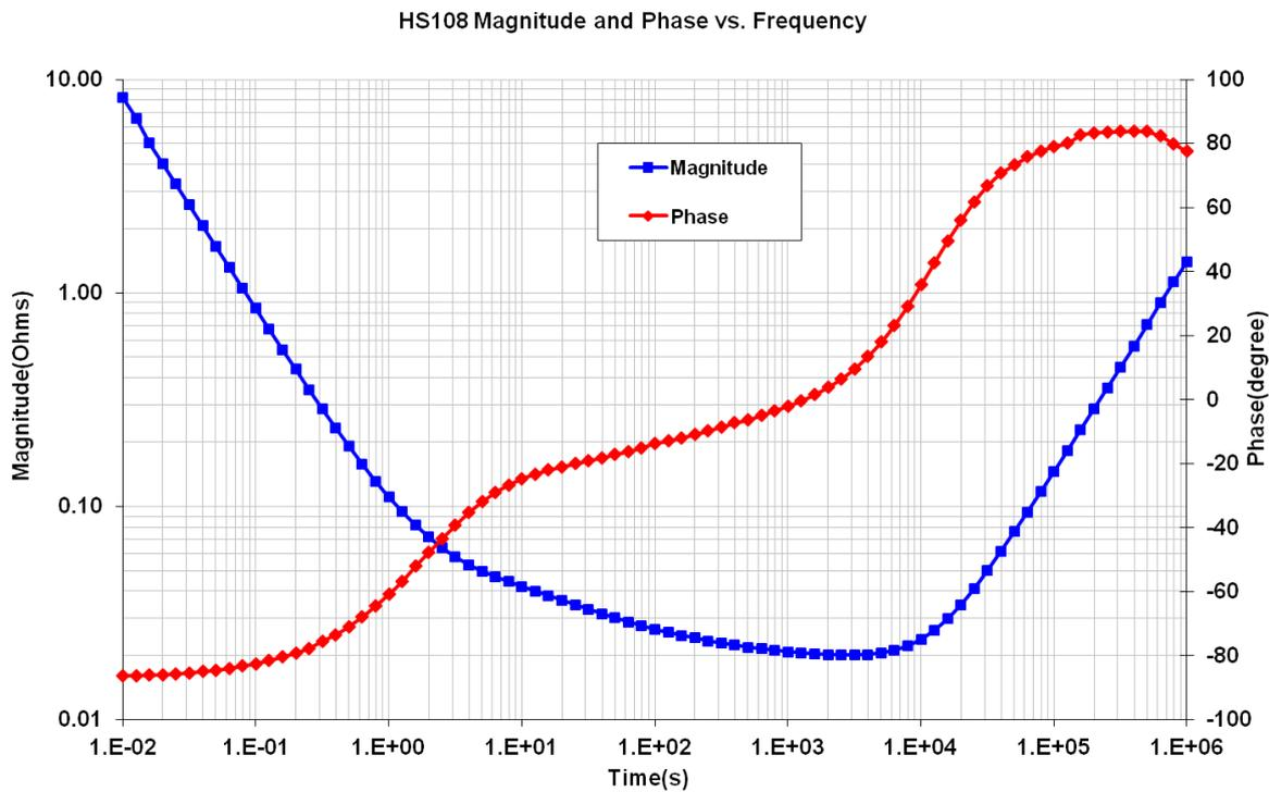
**Fig 8: Frequency Response of Impedance (biased at 2.7V with a 50mV test signal)**
