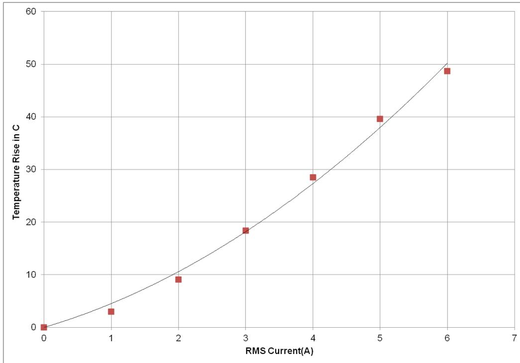
**Fig 12: Temperature rise in HS208 with RMS current**
