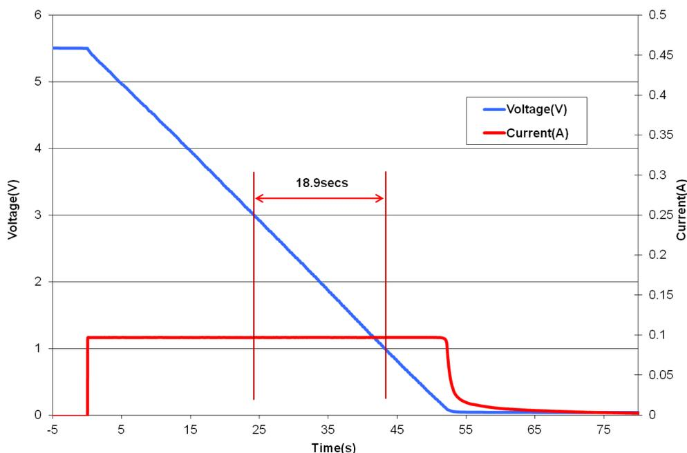
**Fig 2: Measurement of DC Capacitance for an HS208**
