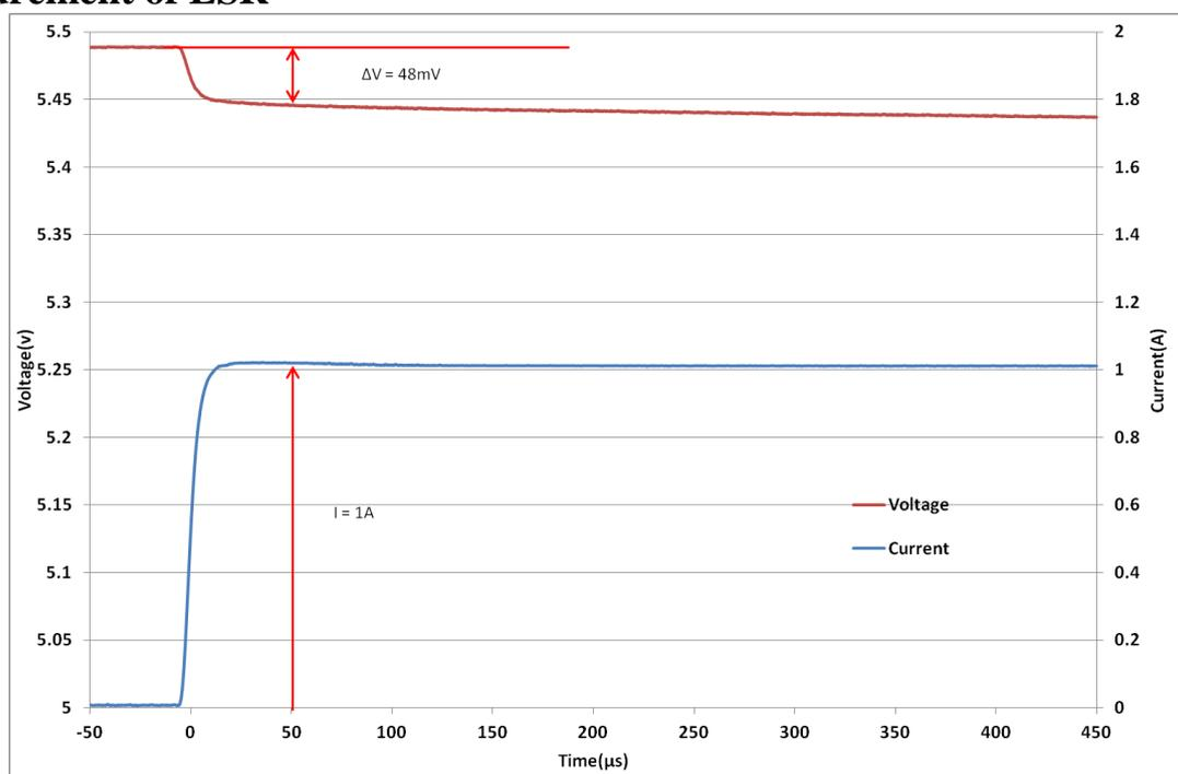
**Fig 3: Measurement of ESR for an HS208**
