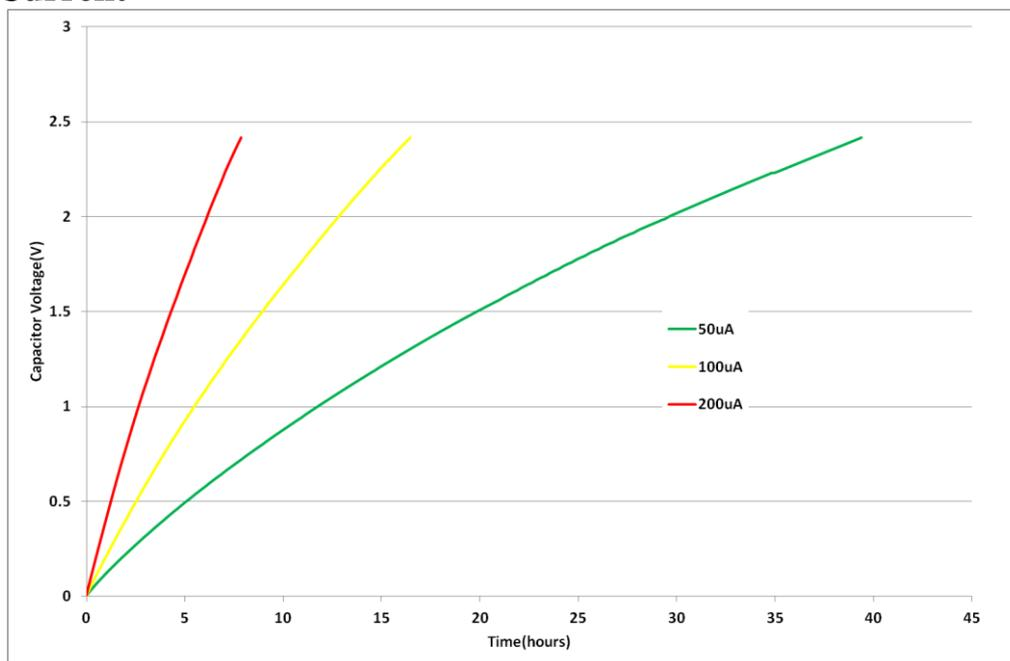
**Fig 11: Charging an HS108 with low current**
