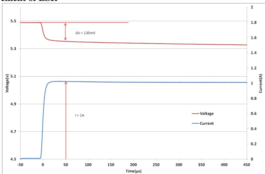
**Fig 3: Measurement of ESR for an HA230**
