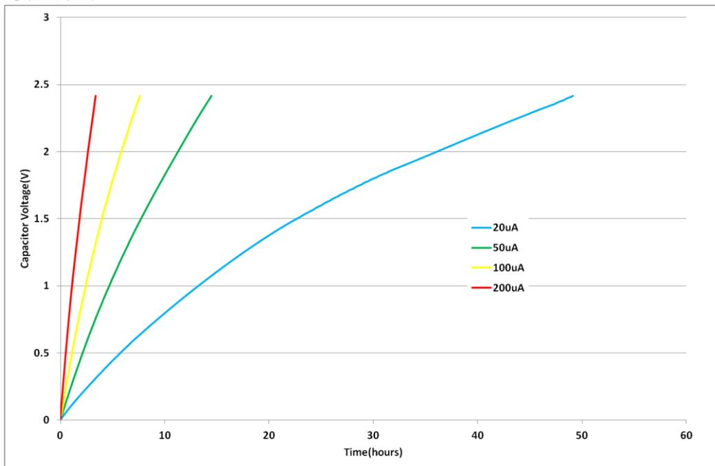
**Fig 11: Charging an HA130 with low current**
