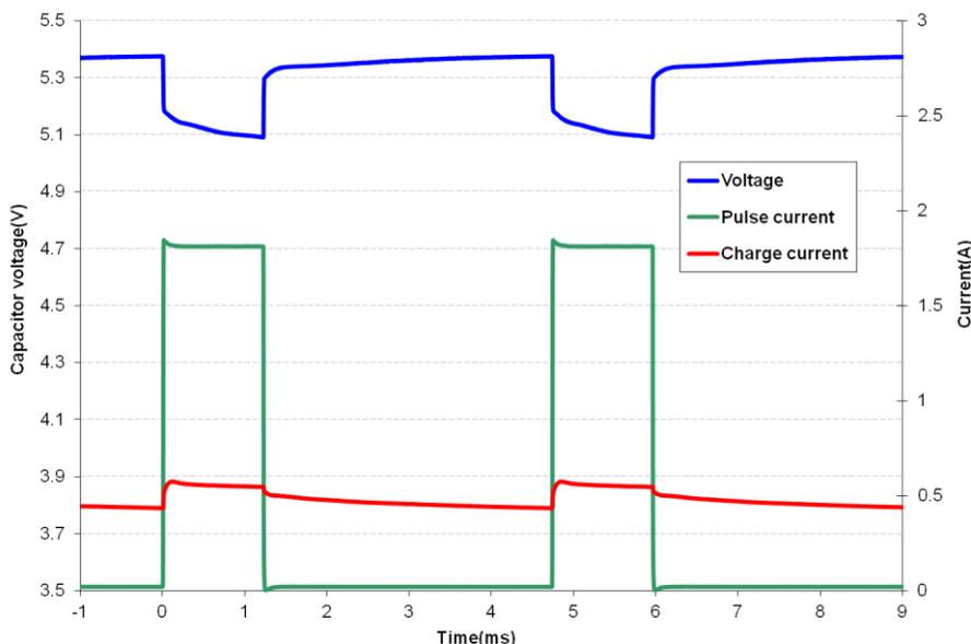
Fig 5 shows that the HA230 supercapacitor does an excellent job supporting a GPRS class 10 pulse train, drawing 1.8A for 1.1ms at 25% duty cycle. The source is current limited to 0.6A and the supercapacitor provides the 1.2A difference to achieve the peak current. At first glance the freq response of Fig 8 indicates the supercapacitor would not support a 1ms pulse, but the  $C_{eff}$  of 26mF coupled with the low ESR supports this pulse train with only ~280mV droop in the supply rail.
