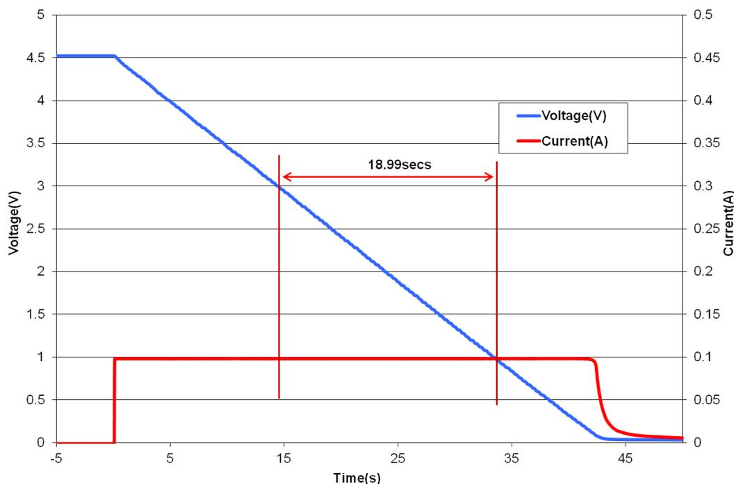
**Fig 2: Measurement of DC Capacitance for a GS208**
