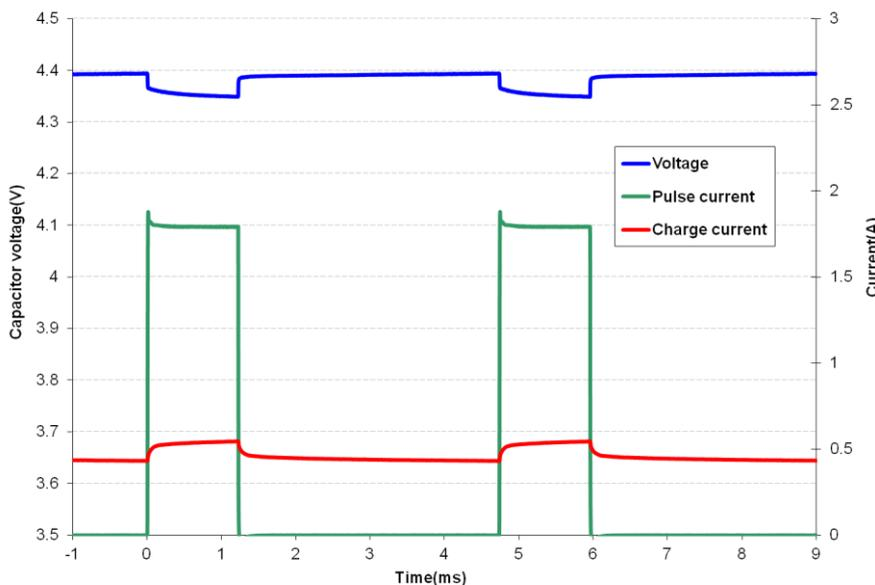
Fig 5 shows that the GS208 supercapacitor does an excellent job supporting a GPRS class 10 pulse train, drawing 1.8A for 1.1ms at 25% duty cycle. The source is current limited to 0.6A and the supercapacitor provides the 1.2A difference to achieve the peak current. At first glance the freq response of Fig 8 indicates the supercapacitor would not support a 1ms pulse, but the  $C_{eff}$  of 58.5mF coupled with the low ESR supports this pulse train with only ~45mV drop in the supply rail.
