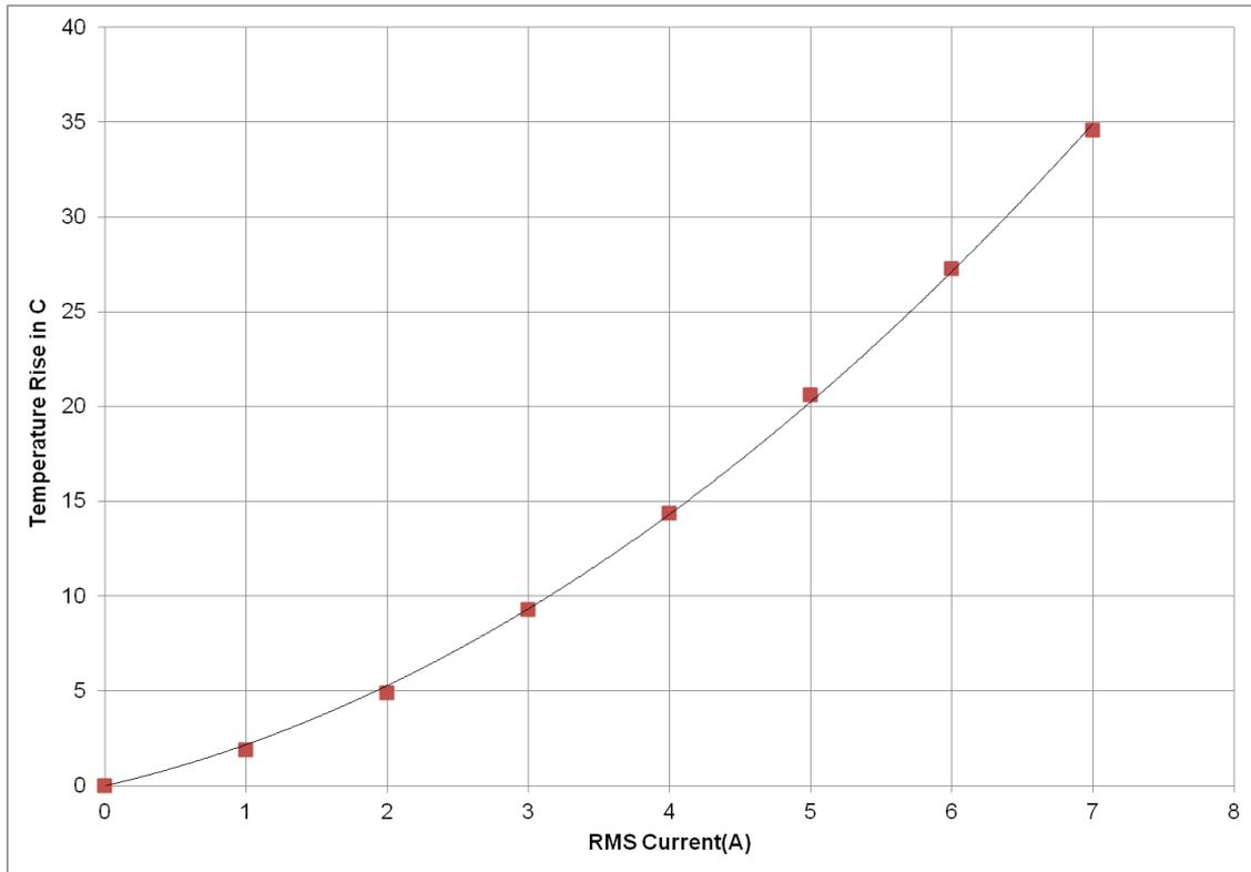
**Fig 12: Temperature rise in GS208 with RMS current**
