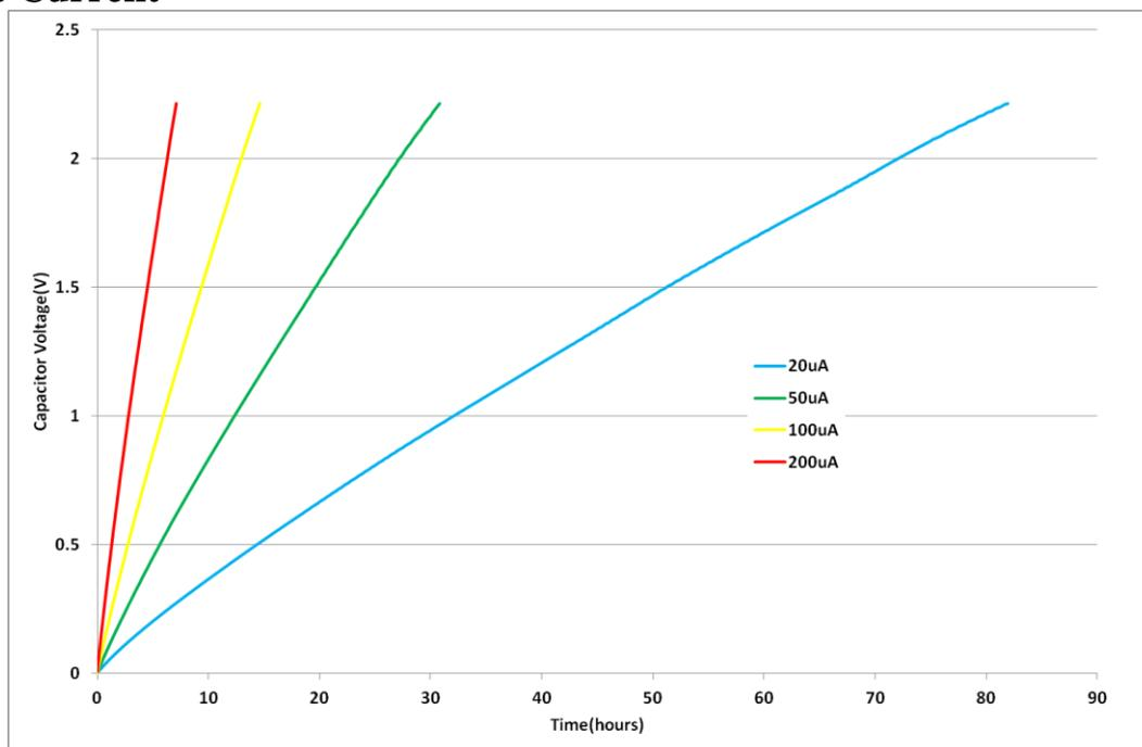
**Fig 11: Charging an GS108 with low current**
