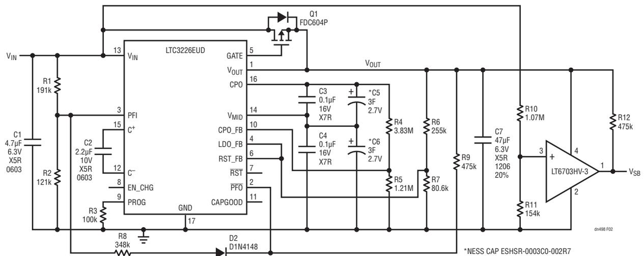
Figure 1. A Typical Power Backup System Using Supercapacitors
