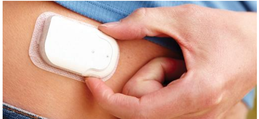
Semi disposable insulin device, with a CAP-XX supercapacitor
