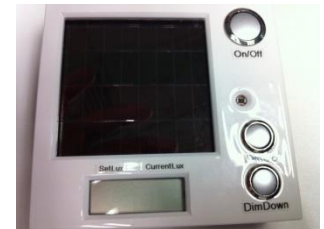
Solar building controls (Schneider "Tango")
