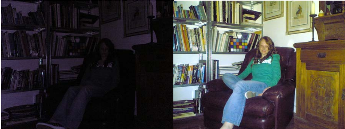
Fig 3: Photos in low light with normal phone (left) and phone modified with CAP-XX supercapacitor-based solution (right)
