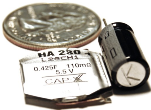
Fig 13: Size comparison between prismatic supercapacitor and cylindrical electrolytic storage capacitor used for xenon flash. The SonyEricsson K800 uses two of these electrolytics; the Nokia N82 uses one of the same size.
