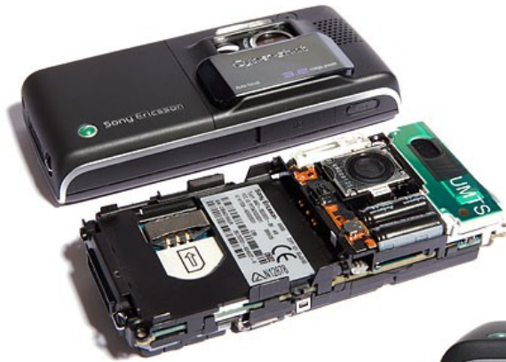
Fig 12: The bulky electrolytic capacitor precludes a thin form factor for a xenon flash solution with adequate light energy.
