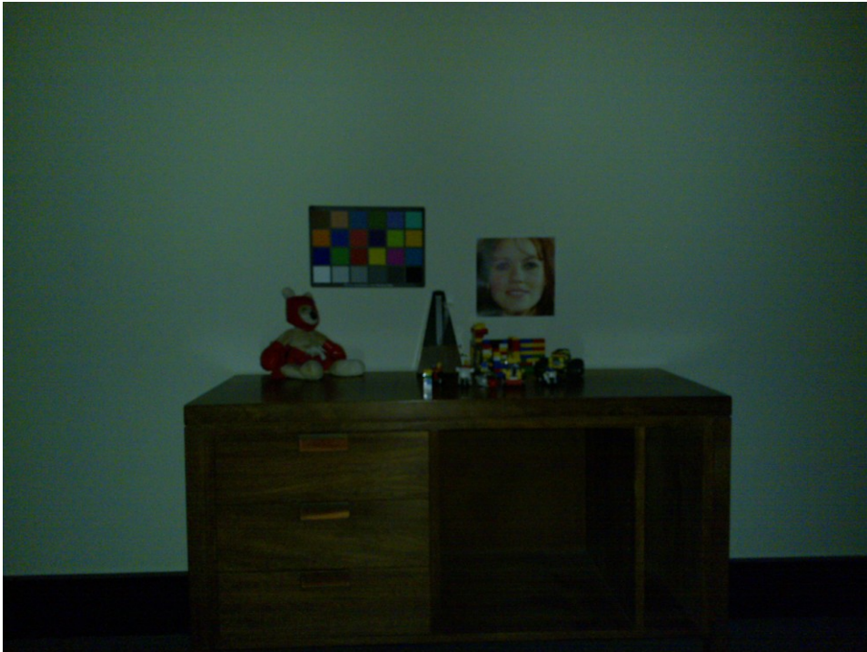
Fig 11a: Test scene shot from 2m in a dark room, using a standard Nokia N96 with 2 LEDs with no supercapacitor support. Note the poor color reproduction from the color chart. There is also a metronome ticking at 1Hz to show blurring due to exposure time.
