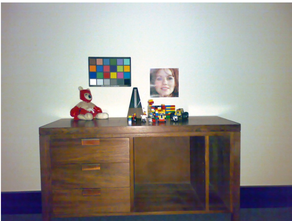
Fig 11b: The same scene as Fig 11a shot with a Nokia N73 modified with a supercapacitor to drive 3 x LEDs at 1A each for a total flash power of 12W. The color chart shows much better color rendition than Fig 11a, and the metronome arm shows less blur from a faster exposure.
