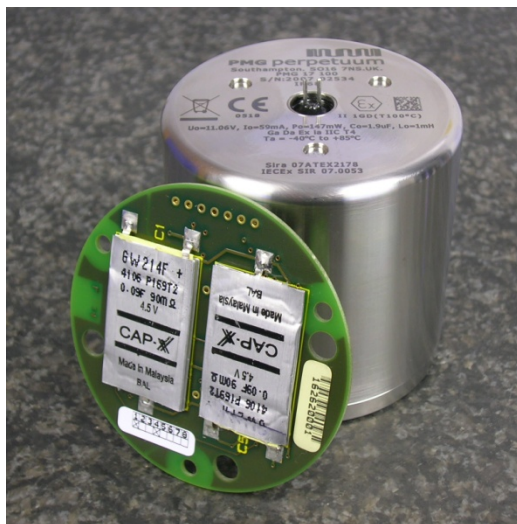
Fig 8: PMG17 Vibration Energy Harvester and Power Conditioning PCB; CAP-XX Supercapacitor with 25c coin comparing size
