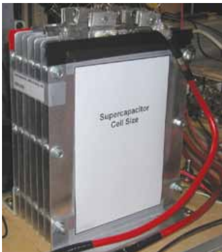
Supercapacitor testing module (14V) for Automotive Stop/Start
